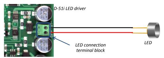
**Note!** All driver connections in this manual are pointed for D-51i LED driver; connections with other drivers should be done similarly.
