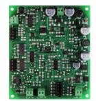
D-41i Driver provides **Pulse mode** operation. Using this mode it is possible to choose one of five current values (0.2/0.6/1/1.5/1.9 A) and select one of four frequencies (0.5/1/2/4 kHz) and choose pulse duration within five values  $(5/10/20/50/150 \,\mu\text{s})$ .
