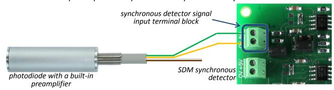
Green cord – to the signal input "+"; Yellow cord – to the signal input "0"
