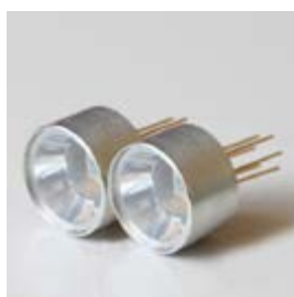
TO-5-TEM-R with a parabolic reflector with a glass cover
